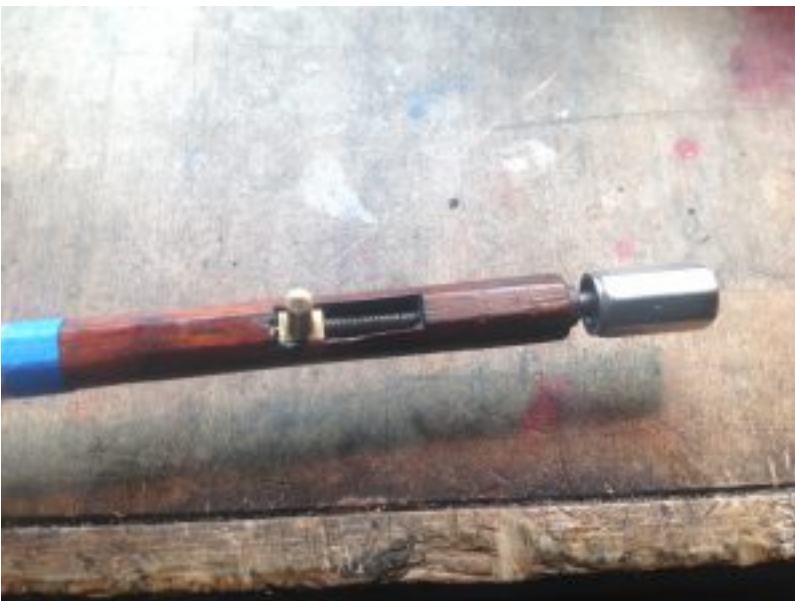
Eyelet positioned in the front of the mortise.
