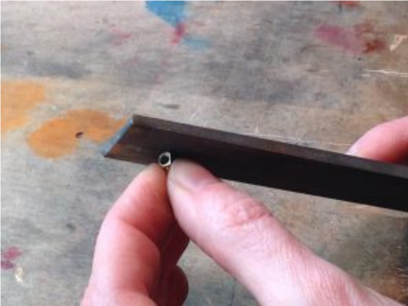
Filing top of the head of the new eyelet.
