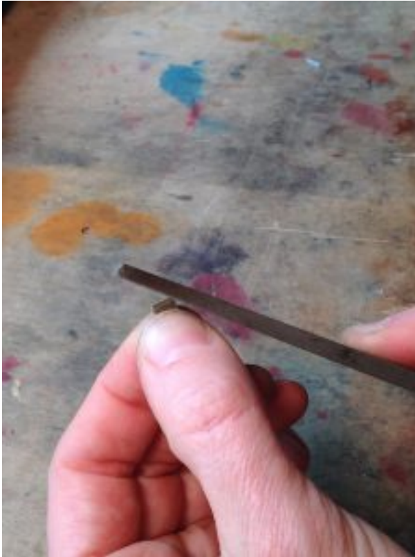
Filing a bevel on the end of the eyelet head.
